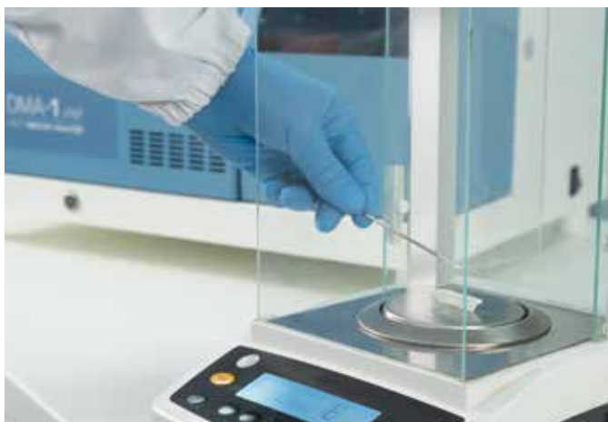
Sample is weighed inside the metal or quartz boat
