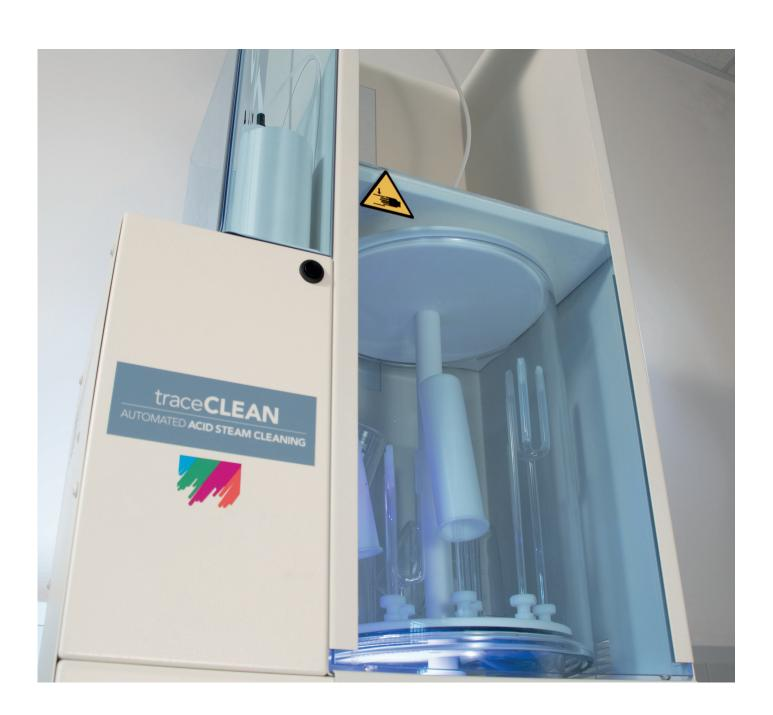
Typical cleaning procedures involve either acid baths or a microwave method to clean digestion vessels, glassware and ICP accessories, both approaches limit productivity and efficiency. The acid steam cleaning process in the traceCLEAN ensures lower blanks, improves your detection limits, without compromising the throughput.
