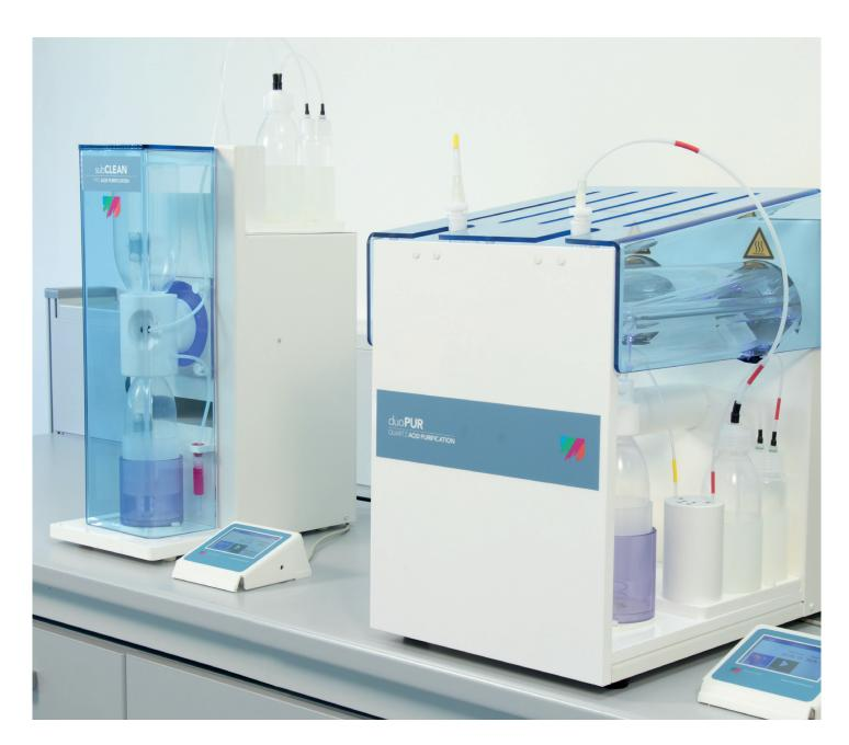
Milestone applied sub-boiling distillation technology in the duoPUR and SubCLEAN. The duoPUR has two quartz purification units and allows the purification of the most common acids such as HNO<sub>3</sub> and HCl, while the SubCLEAN has a single PTFE-TFM purification still, allowing the purification of HNO<sub>3</sub>, HCl and HF too.
