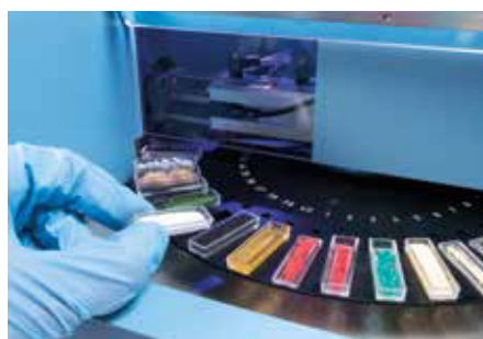
Sample boat is placed into the autosampler
